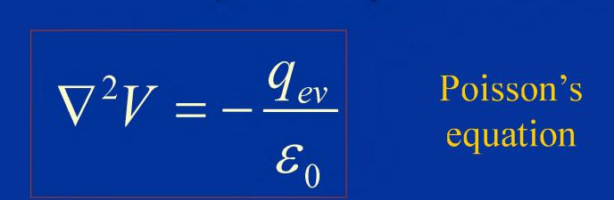
$\Rightarrow \nabla^2$  is the *Laplacian operator*. The *Laplacian* of a scalar function is a scalar function equal to the divergence of the gradient of the original scalar function.
