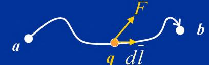
$$W_{a \to b} = -\int_{a}^{b} \underline{F} \cdot d\underline{l} = -q \int_{a}^{b} \underline{E} \cdot d\underline{l}$$
