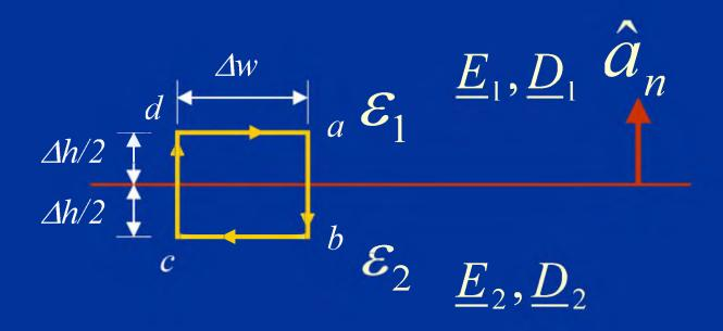
**Boundary Condition on Tangential** Component of E (Cont'd)  $\hat{a}_{s}$  = unit vector perpendicu lar to path *abcd* in the direction defined by the contour  $\hat{a}_t = \hat{a}_s \times \hat{a}_n$  = unit vecto r tangenti al to the boundary along path
